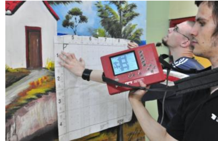
Ferroskan: reinforcement location
