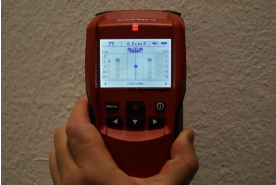
Figure 4.3: Detecting of ferrous metal in a concrete column with the use of HILTI PS 50 Multidetector
